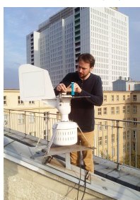
Test setup PPS and Burkard trap for comparative measurements. The orifice of the Burkard trap and the PPS are orientated equally
